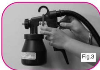
Completely close adjustment screw (4) by turning this clockwise as far as it will go. Whilst pulling the trigger, begin turning the adjustment screw anti-clockwise until the volume of paint you require is obtained. If the paint spray is too wide or contains too much paint turn the adjustment screw clockwise again. Once the correct spray pattern is obtained you are able to commence spraying.
