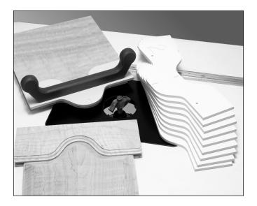
**Raised Panel** - Panels are usually made of 5%" or 3/4" thick stock. The panel is made 1/2" wider and 1/2" taller than the opening made by the inside dimensions of frame (not the cabinet opening.) This allows for 1/4" tongue insertions into the stile and rail grooves on each of the four sides.
