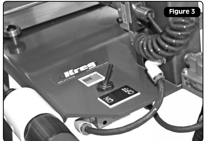
Throw cylinders independently or all at once with the master switch
