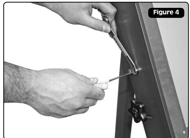
Re-tighten locking nut once complete.
