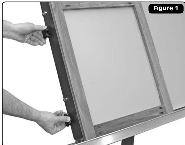
Place workpiece into alignment with squaring fence
