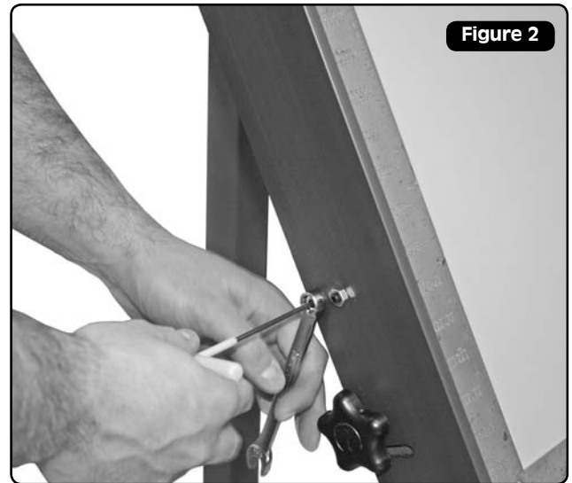
Loosen locking nuts with hex wrench, and adjust the set screws with an allen wrench to square fence.
