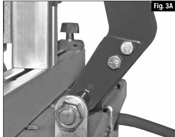
Handle with bolts, washers, and nuts properly installed.
