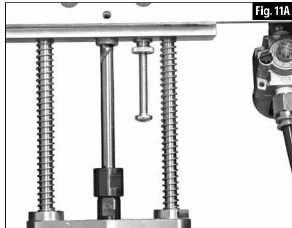
The Depth Stop Adjustment Screw limits travel of the Drill Bit.
