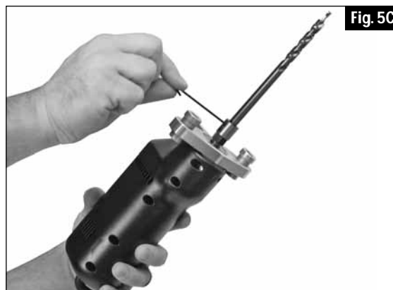
The Drill Bit is held in position with set-screws in the Drill Adapter.
