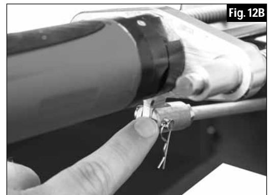
Disconnect the Connecting Rod to remove the Air Drill Motor from the Guide Rods.
